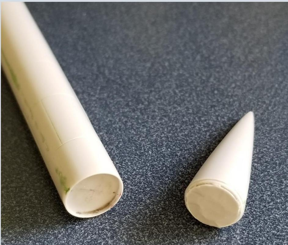
The nose cone required little work to fill or shape. In fact, once attached to the body tube, it was only necessary to sand it lightly to smooth the joint between the parts.
