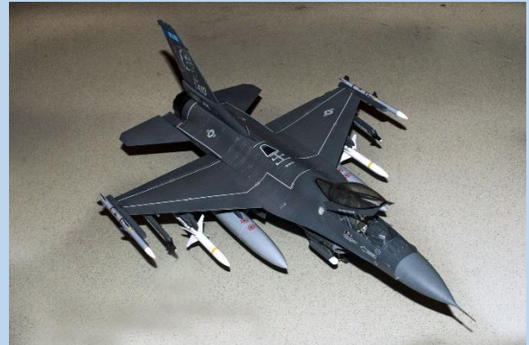
Caracal Decals. Have Glass Scheme Tamiya paints mixed for Have Glass. Didn't achieve desired results so over sprayed with MRP Paint Have Glass paint, then Tamiya clear gloss for final result. Tamiya paints for detail painting Master Model brass pitot tube
