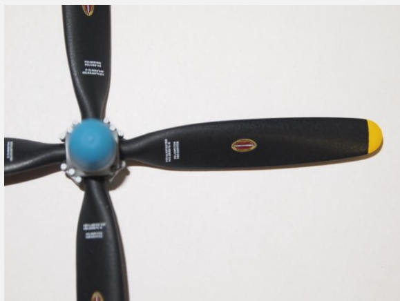
Hamilton Standard 13' diameter blades utilizing the most common white data. The image doesn't do justice to the logo.
