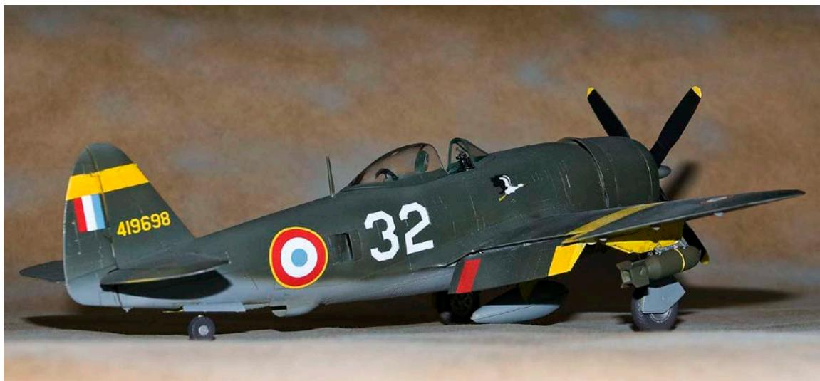
Construction is simple and pain free, the interior is nicely detailed only needing photo-etched seat belts to complete it. Tamiya provides a decal for the instrument panel that, if applied with hot water, looks fantastic. A note for P-47 novices, the interior color was a dark green similar to FS 34092. I used Gunze Sangyo's version of this color, H-302, but has this paint line is no longer imported into the States. Model Master also includes this color in their paint line.
