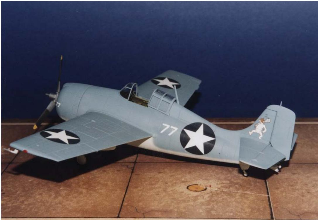
The wing-to-fuselage fit is excellent and little or no filler will be needed. Assemble and paint the Pratt and Whitney R-1830-86 Twin Wasp engine. I used “gunmetal gray” on the cylinders and light gray, FS-16320, on the crankcase. A wash of gloss black will bring out the details of the powerplant.
