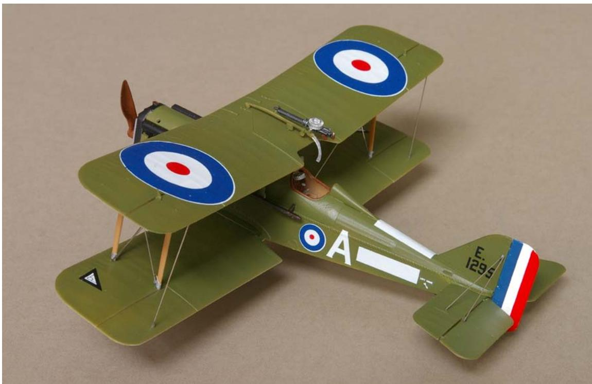
Glue the interplane struts to the bottom wing with white glue. When they have dried, flip the model over and careful position and glue the top wing onto these struts. Support the wing with  $\frac{1}{2}$  oz. paint bottles until the adhesive has set up. The cabane struts can now be cemented into place.
