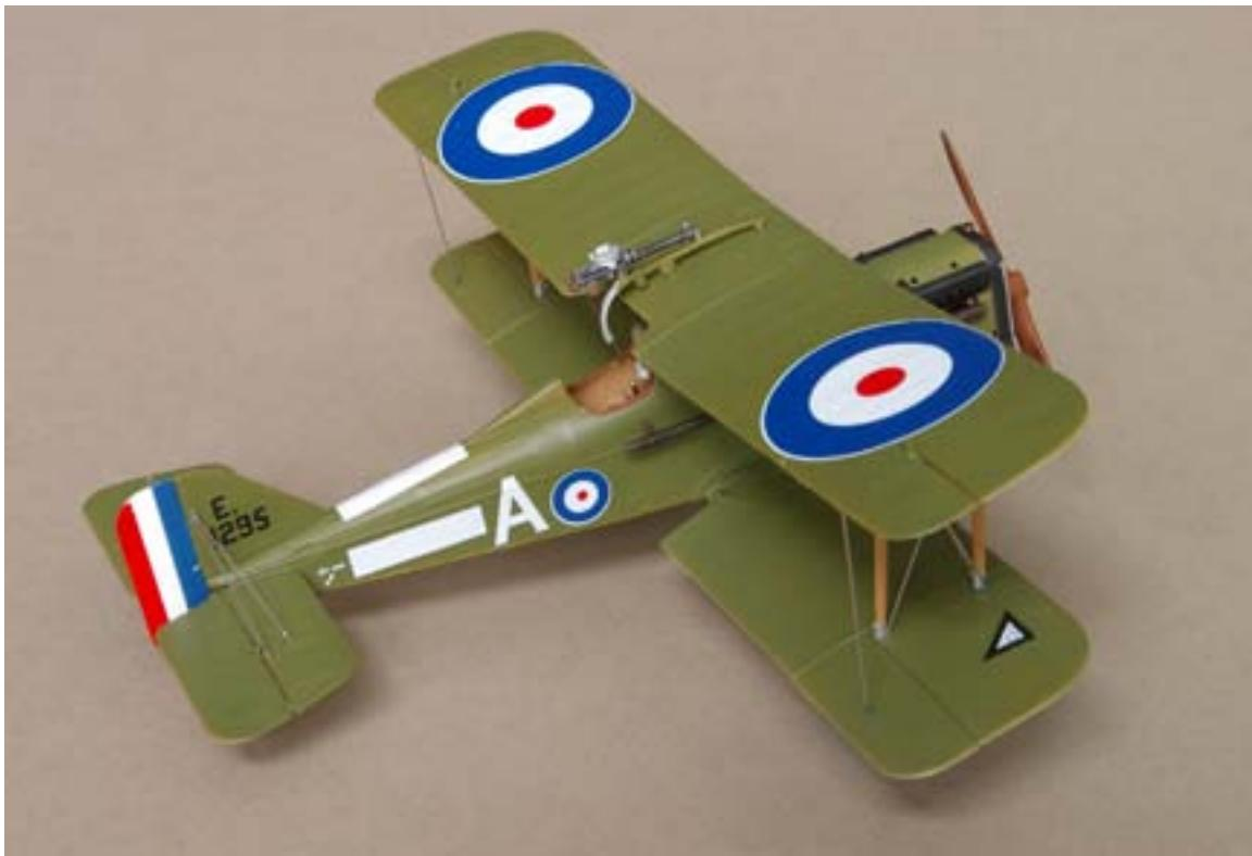
Trap the finished cockpit into the fuselage and glue the right and left sections together making sure the floor is level. Attach the upper forward section of the fuselage, cylinder head covers and radiator into place. The horizontal stabilizer, elevators and lower wing can also be glued to the fuselage at this time.
