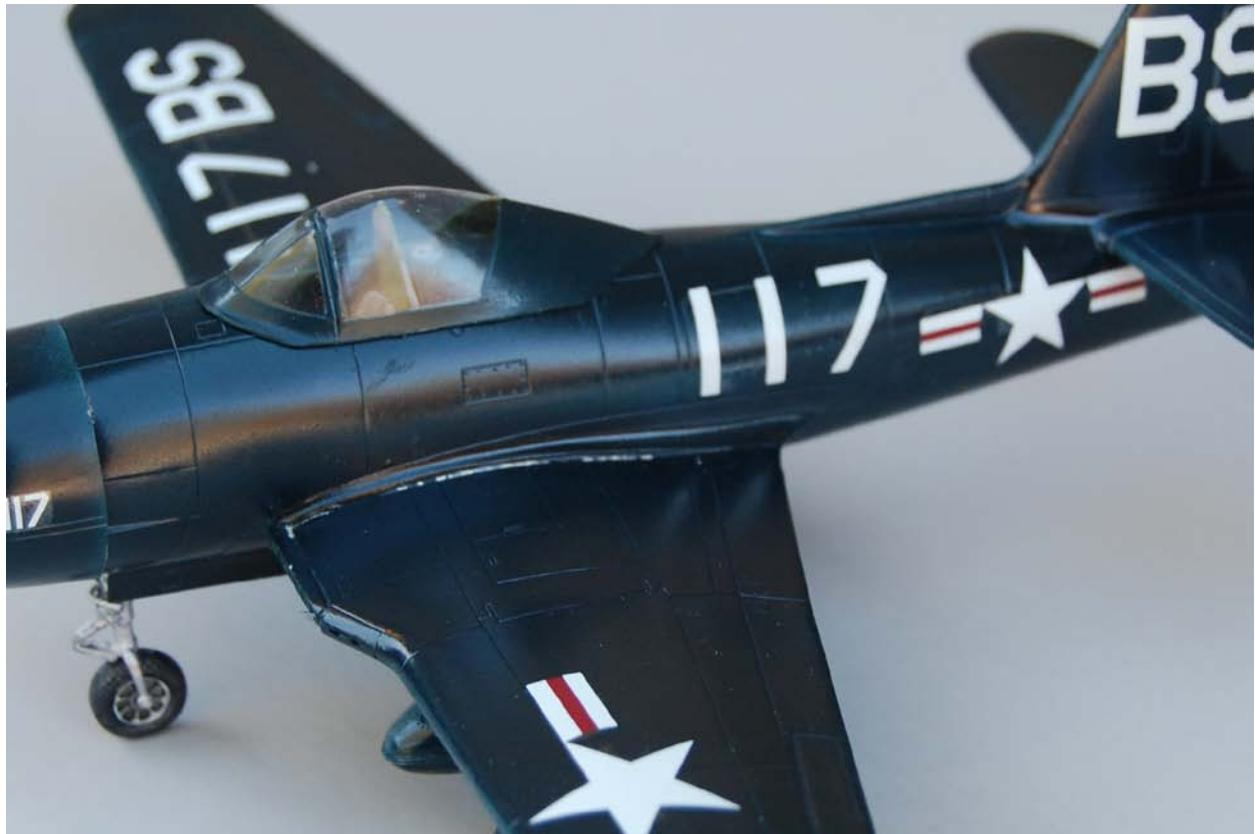
I then masked off the canopy frame and painted the frame Model Master Interior Green prior to putting on the final coat of Dark Sea Blue. Also I got the wheel well doors and auxiliary fuel tanks ready for painting. I drilled some holes in the fuel tanks and mounted them on some toothpicks. I attached the tank pylons to the wing at this time
