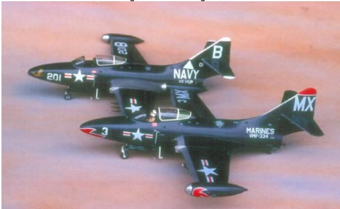
You will find the fuselage goes together easily enough, but some minor filling will be required. I used cyanoacrylate for filling the seams, notably on the forward fuselage and the length of the underside. Just a little sanding and it's onto the next step.
