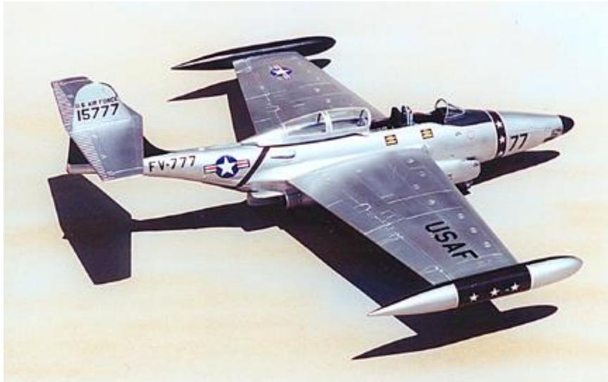
F-89Bs' and the first 40 or so F-89Cs' had an external counter balance system on the horizontals. These are easily seen as they form several horn shaped loops on the top and bottom those surfaces. After an internal fix was implemented for the F-89C, many F-89Bs' were also retrofitted. As this was the only major external difference, you can build most F-89B or C options that may crop up on after market decals, just check your references!
