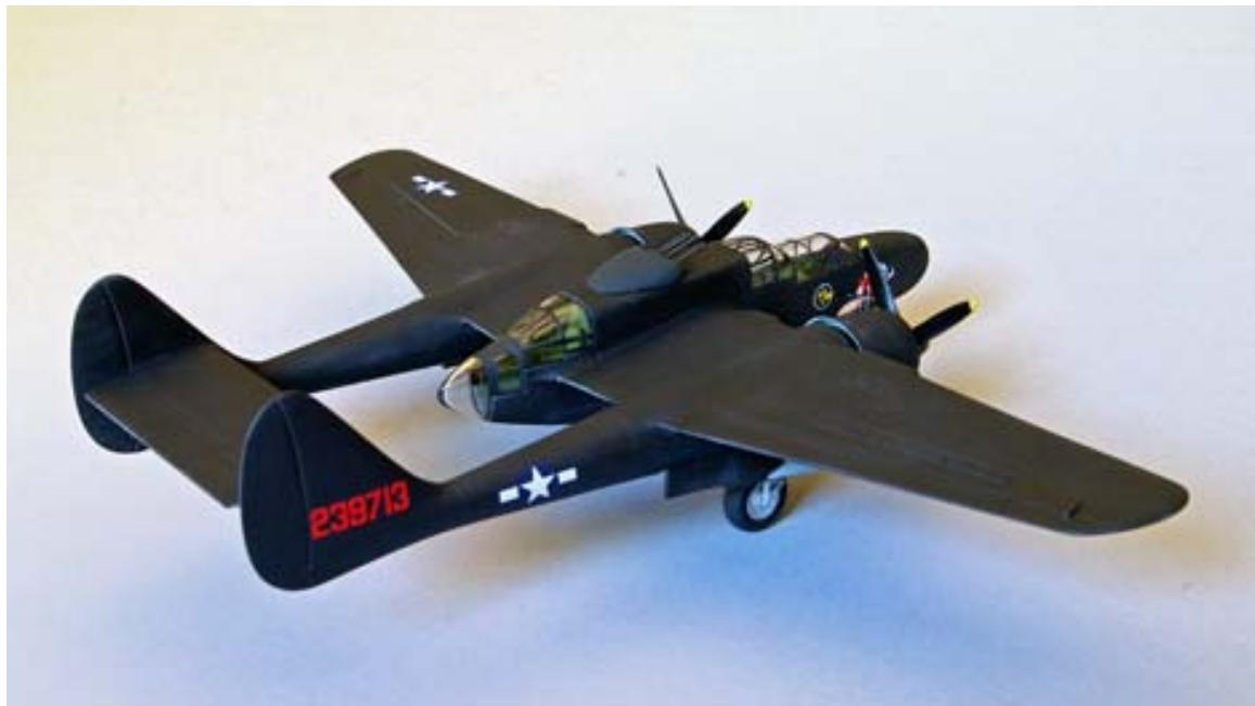
Additionally, fill the engine cowlings with BB’s and secure them with white glue and set these parts aside to dry. Glue the wings to the fuselage. The joint here will require an application of putty.
