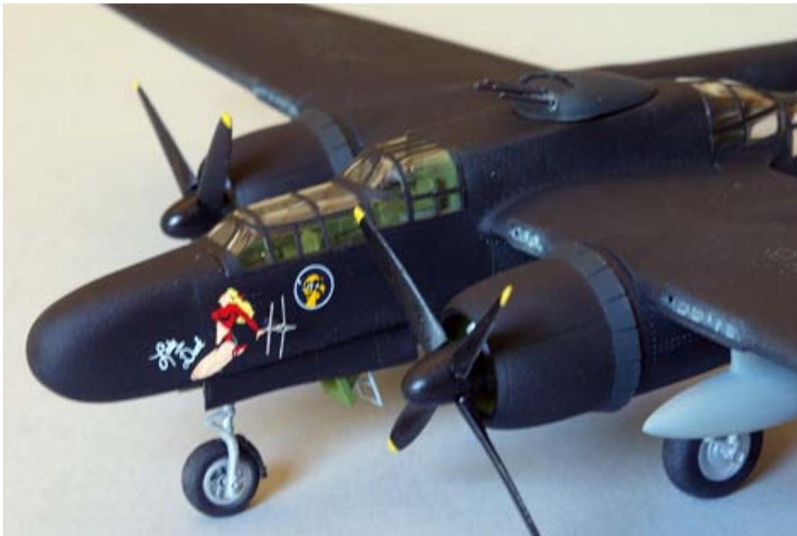
The extensive framing on the “greenhouse” canopies is somewhat of a daunting painting task but can be made simple by first masking and painting all of the vertical braces and when dry, mask the horizontal frames and then paint them.
