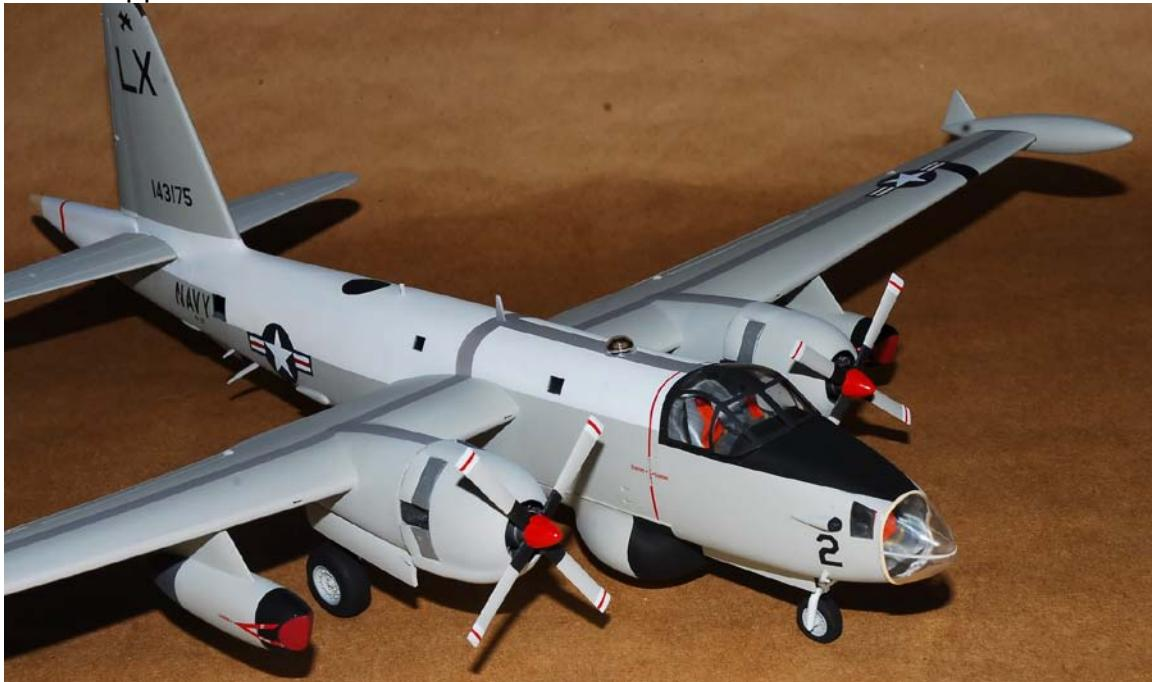
Since this model was for the Glenview Hanger One museum project, I painted the aircraft in the 70s scheme of flat light gull gray on the lower fuselage, horizontal stabilizers, vertical stabilizer and wings. The top of the fuselage is flat white. I used historical photos of the aircraft to duplicate the paint job. With the fuselage painted and sealed with a coat of Future, I set the model aside to prepare for the decals.
