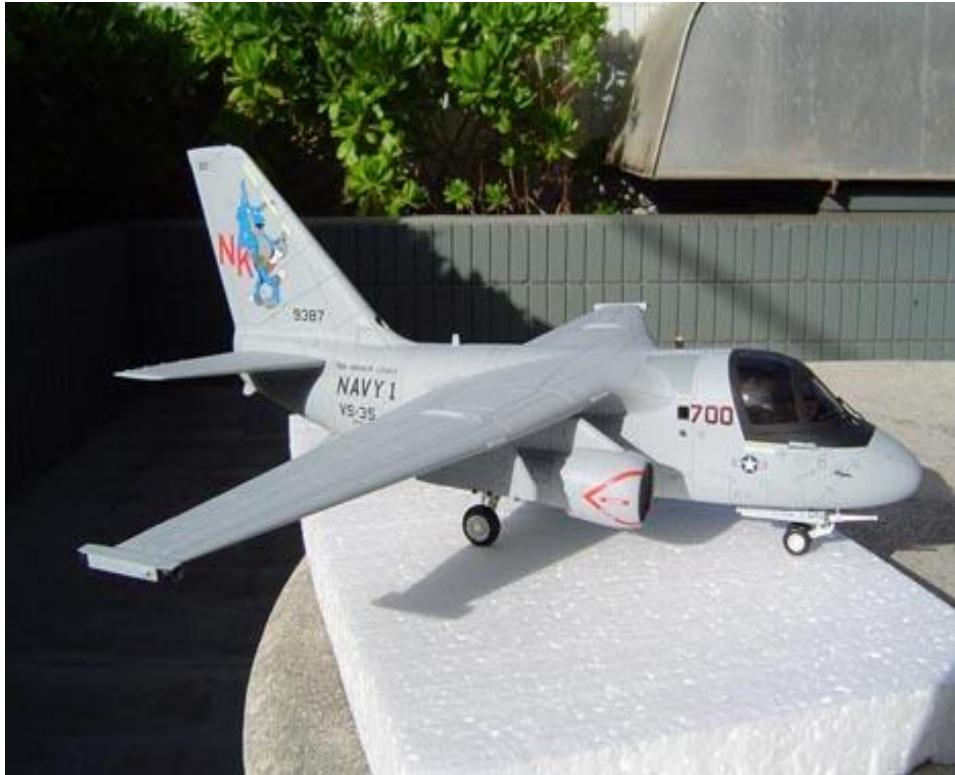
I hacked off the antenna on top that looks like half a boomerang and I didn't glue on any of the other antennas (parts #41 & 103). The MAD boom was also left out. The model also needs some weights in the nose or else it will sit on its butt. You can also use the tail hook to prop it up.
