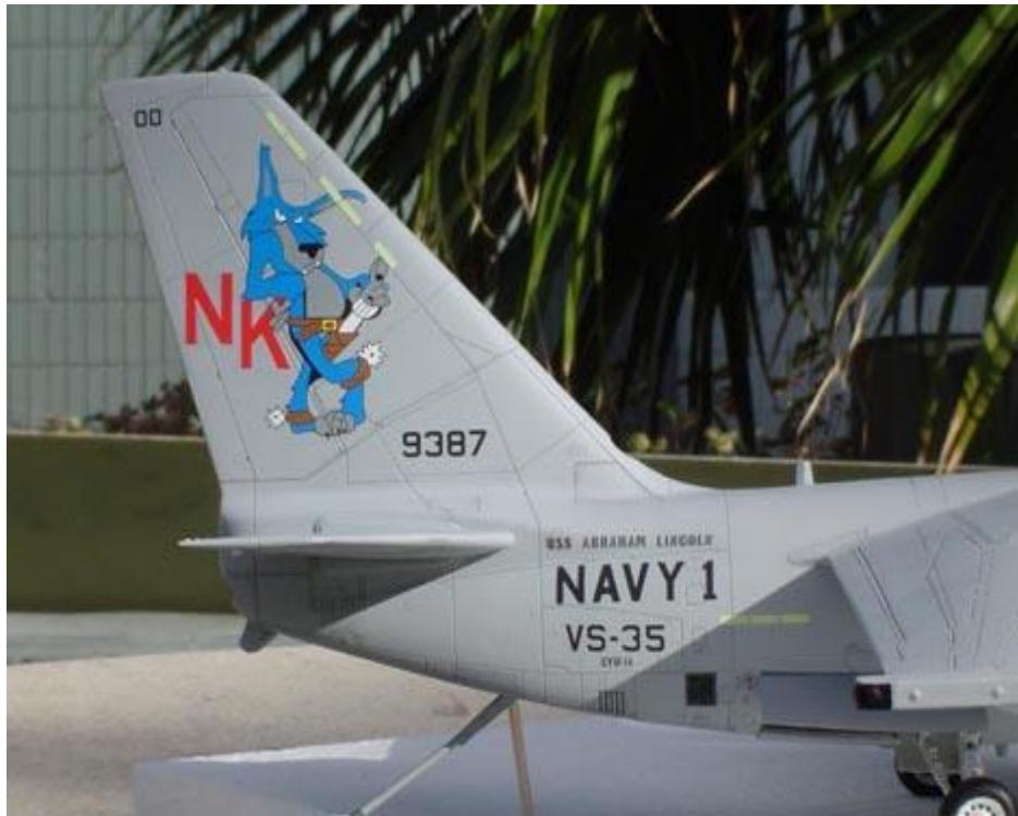
The middle 'slime light' on the tail was positioned exactly perpendicular to the panel line underneath the Wolf's left ear. This is an important reference point because the next decal is the Wolf, which fits perfectly. Be sure the light on the other side is in the exact same place.
