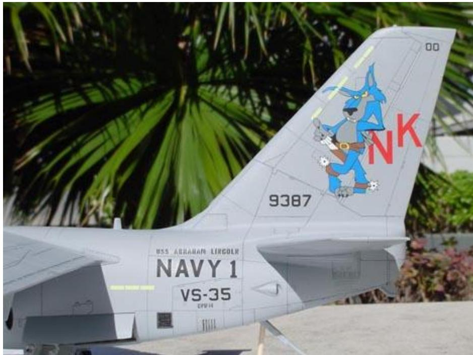
The 'slime light' decal was applied first because the Wolf's finger was painted over part of the light as you will see in the photo of the real NAVY 1. Positioning of the light is most important and must match the other side. The Superscale fit was good as you can see the foot didn't go over the wing fold.
