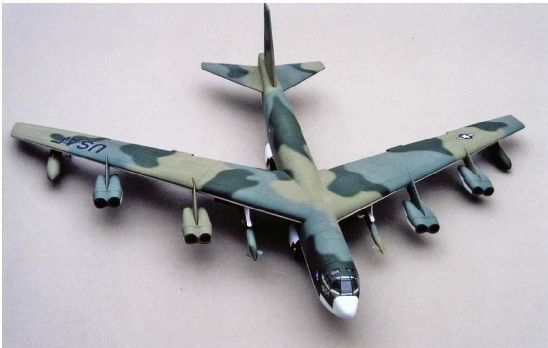
Captain Phillips recalled that the underside of all the aircraft in his squadron were painted in "anti-flash" white, FS-17875, as were the radomes on the nose and tail. (The white was to reflect the flash and heat from a nuclear blast directed toward the bombers.) The rest of the aircraft was painted in the standard Strategic Air Command's three-tone camouflage with a "hard" demarcation line separating the underside color from those on the topside.
