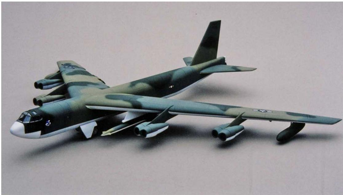
The "H" model was the last of the Boeing Company's 744 total production of B-52 Stratofortresses. The "H's" appeared much like the earlier "G's" but were easily recognizable by their eight larger Pratt and Whitney TF-33 turbofan engines.
