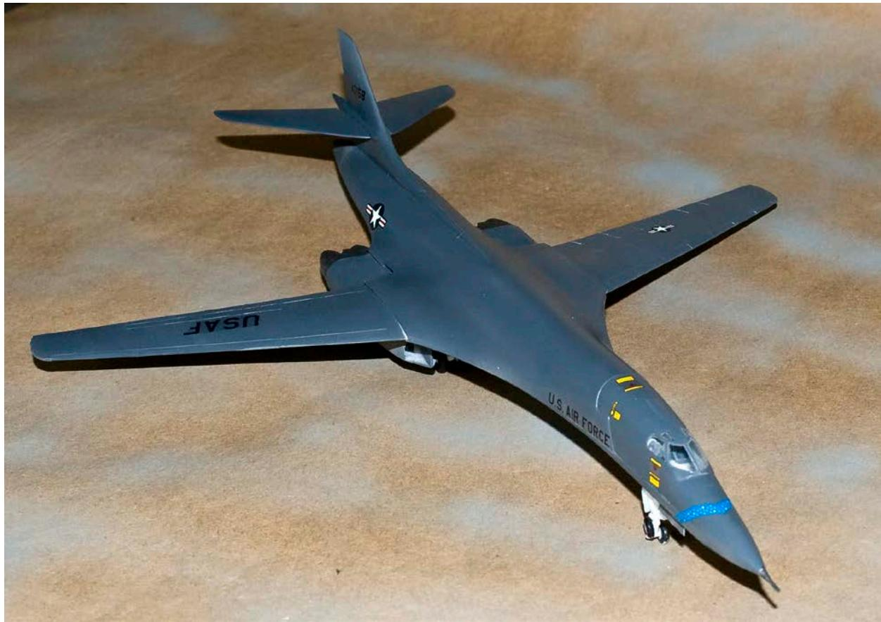
I did not use a base coat, but used Model Master Acryl Gunship Grey 4752/36118. I applied several light coats to insure I had good coverage and eliminated the chance for any runs. Even though the B-1A was painted in white, I decided to paint in the color of a B-2B Bomber. I then painted the exhausts Titanium from a spray can after it was decanted, with a brush. After letting the paint dry for a few days, I covered it with a few light coats of Future.
